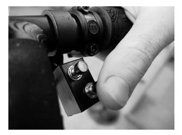
More than one button push in either or both directions does no harm, however the mechanism responds only to the first button push after the last shift is completed. All excess button pushes are forgotten.
