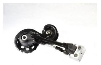
The chain tensioner resides under the rear cogset and provides light return spring tension that assists with guiding the chain during the swing-gate shifting action.
