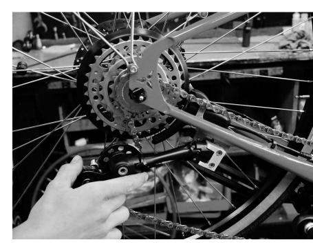
Lubrication can be performed with a lightweight lubricant on the various pivot points of the chain tensioner. If spring action appears stunted and lubrication does not help, a visit to an authorized Shift-E service center is in order.
